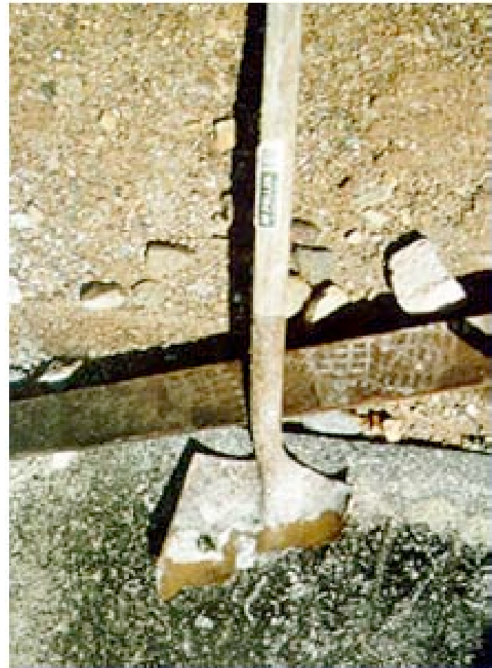
Photo 5: According to EPA documents, workers once inadvertently left a shovel standing in the green liquid flowing from one of the mine portals. The next day half of the shovel had been eaten away.
