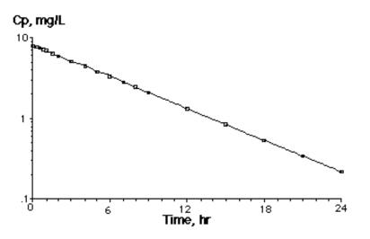
A plot of this same data using a log scale on the y-axis results in a straight line.
